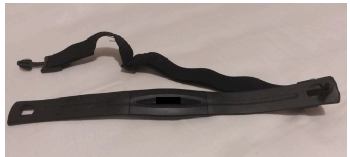
Figure 1: The heart rate monitor chest band.
